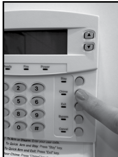
Test your alarm system each month to ensure it is working properly.
