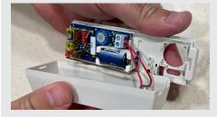
One of the most common yet overlooked maintenance tasks is changing the batteries in your security sensors. Making sure your sensors have fresh batteries can help keep your system working reliably.
